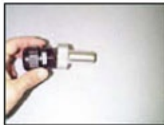
Push the fibre through making sure it extends past the tip of the head.
