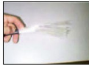
Inspect the fibres making sure none are cut or damaged.
